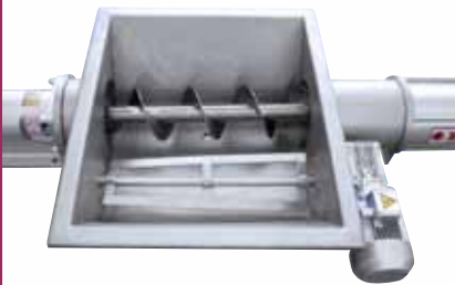
Pump type TLS with paddle bridge-breaker for transfer of whole grapes-fermented grapes
